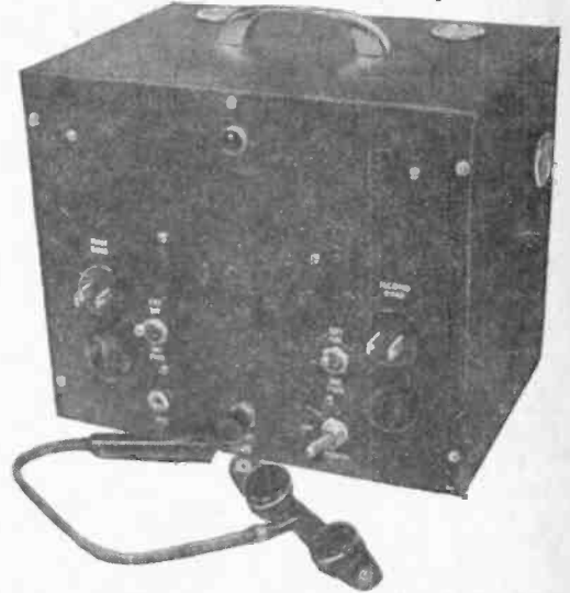
Front-panel view of telephone switch remote control unit. Note circular vents in cabinet. Throat microphone is in foreground.
