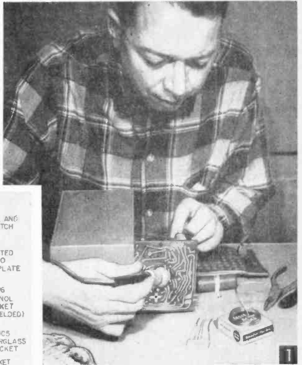
Many printed sets are vertically mounted in cabinet and slide out for quick circuit repair. Note that a fine-tip pencil iron, not over 40 watts, is used to prevent wiring damage.
