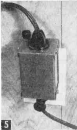
A-C line filter plugged into outlet, with TV set plugged into top. Other half of outlet can be utilized.
