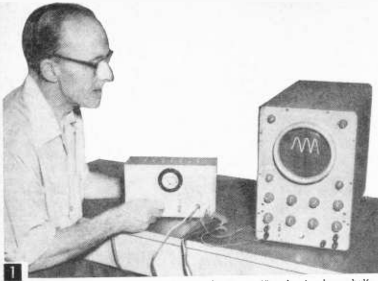
1 Oscillogram pattern of a full-wave, battery charger rectifier showing lower half-cycle, (lost in Fig. 4) inverted and above horizontal centerline, indicating it is being used.
