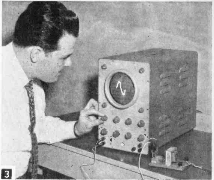
Testing the completed oscilloscope with a small step-down filament transformer. The sine wave shown in the above photograph is one cycle or two alternations of the 60 cycle current.
